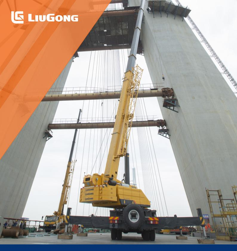
Main Boom49 mJib17.5 mMax Boom Length (Main Boom+Jib)66.5 mMax Lifting Capacity75 TCounterweight16T (2.7T fixed+13.3T fixable)
